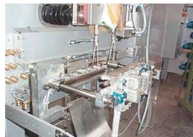
The crimpers in hose packaging machines often reach temperatures of +160 °C and above in continuous operation. The iglidur® plain bearings meet this requirement and are wear resistant.
