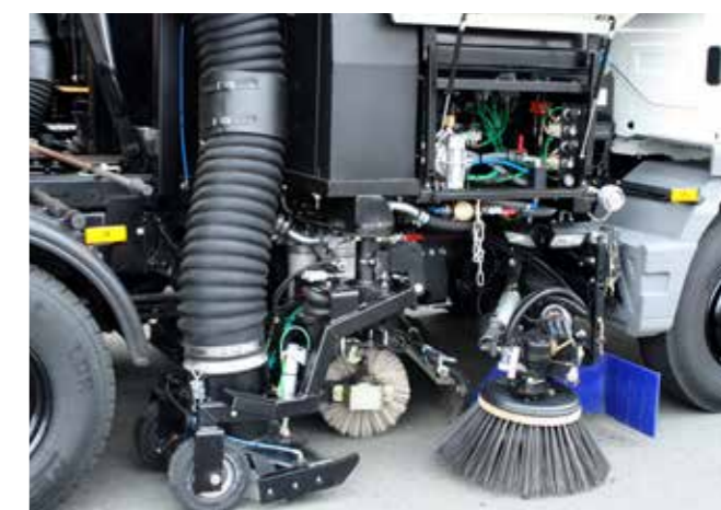
To ensure the long-term durability of the sweepers, the company decided to use lubrication free and thereby maintenance free polymer plain bearings.
