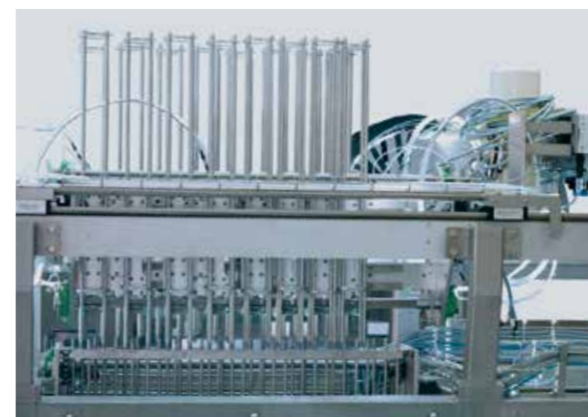
Two longitudinal and one rotary motions can be combined with lubrication free iglidur® bearings in the tightest installation spaces.
