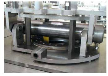
The lubrication free iglidur® PRT slewing ring bearing masters this job brilliantly, is lighter and in terms of purchasing is cheaper than a comparable metal rotary connector.
