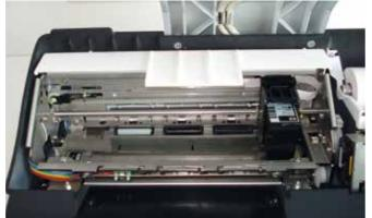
attached using igus® clip bearings.
