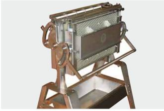
Easy-to-clean and low-cost iglidur® clip bearings and iglidur® flange bearings are used in a honeycomb.
